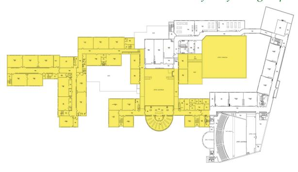
The picture shows the areas of the roof (in yellow) that will be replaced in the proposed project. This section of the roof has been on since 1996-97 and has served us well for seventeen years. The sun and temperature change are the real enemies of flat roofs; we are beginning to experience leaks as the old roof membrane becomes less resilient and expands and contracts. The most serious leaks have been over the small gym and the high
